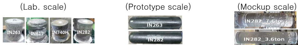
Fig.1 Photograph of manufactured ingots by using the VIM+ESR process for HSC rotor
