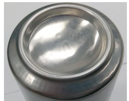
Figure 2. Real can shows wrinkle occurrence
